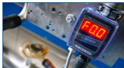
DeLaval flow indicator FI5-D – continuous display of milk flow and yield
